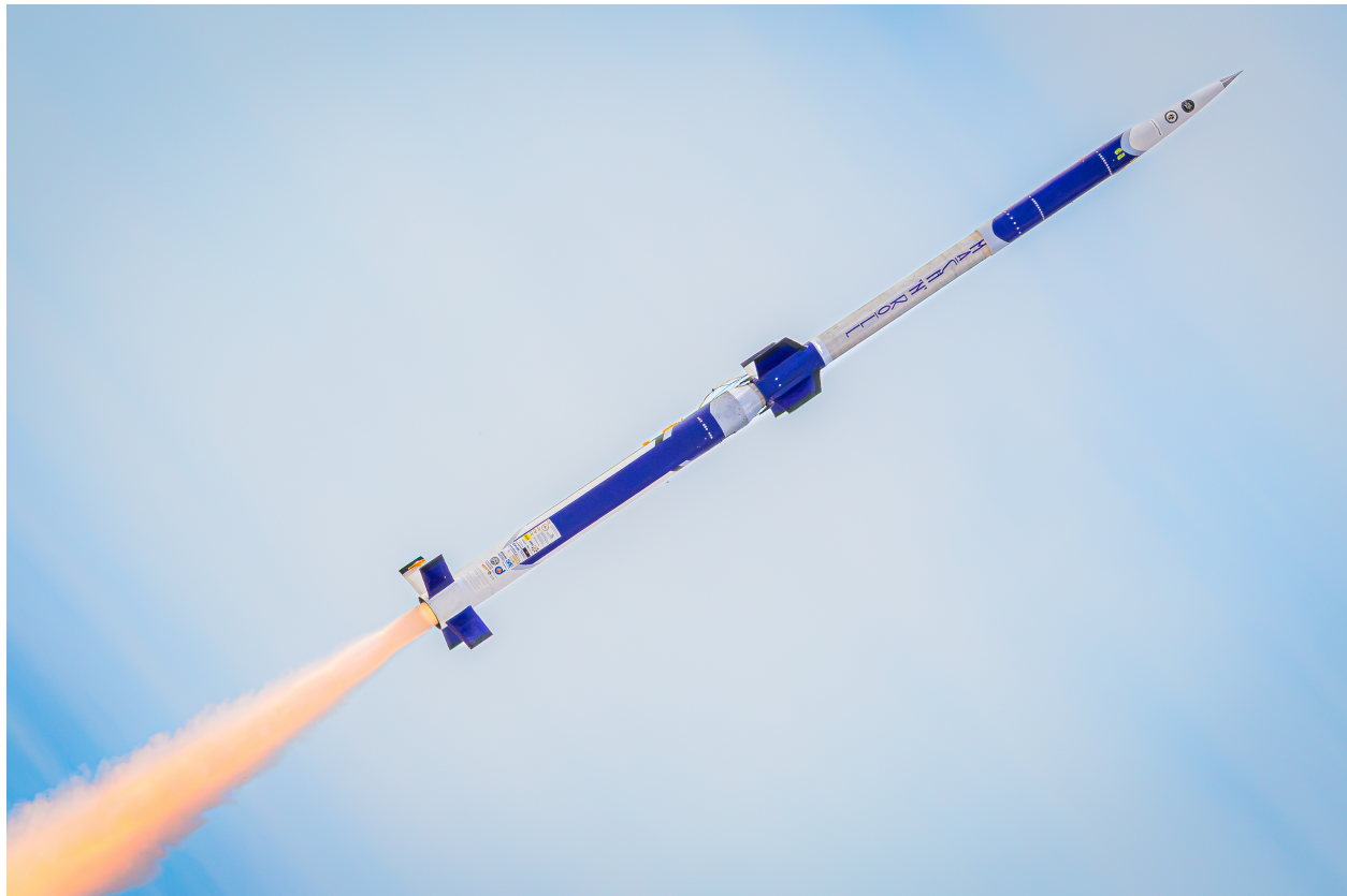
Nominal flight of Mach 'N' Roll (17 ft, 283 lb, two-stage), launched July 2026 to a 31,850-ft apogee
